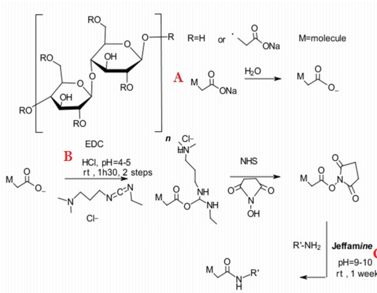
Cellulose is first dissolved in water(A). EDC and NHS are added all at once to prepare the intermediate ester(B). The reaction must be carried out on the carboxylate ion, but because NHS is not very stable and less reactive in a basic or neutral environment, the reaction is carried out at pH = 4-5. Since the intermediate is unstable, the reaction is not prolonged. In a second step(C), the reaction with Jeffamine (primary amine) is more effective in a basic environment.
